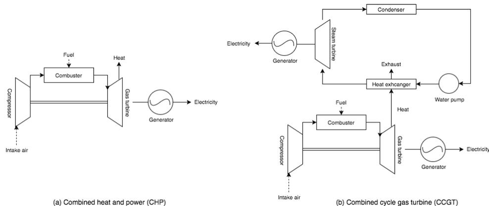
**Fig. 1** Schematic diagrams of (a) CHP system and (b) CCGT system
