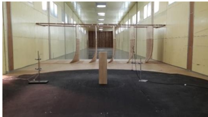
Fig. 4 The building model and the vane system set-ups
