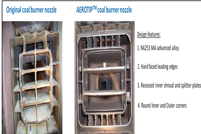
Figure 5: Original coal burner nozzle and AEROTIP™ nozzle
