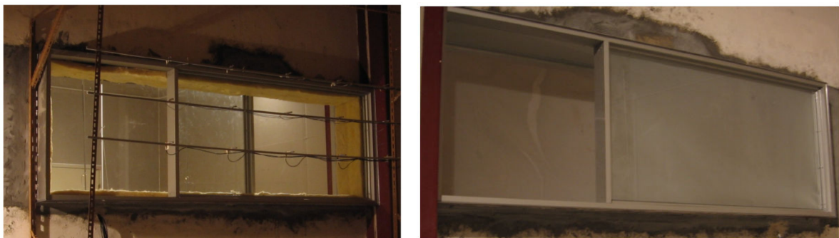
Figure 4: Laboratory Testing Scenarios: Sound Absorption Material on 4 Sides (Left) and Micro Perforated Absorber onto Panes (Right)
