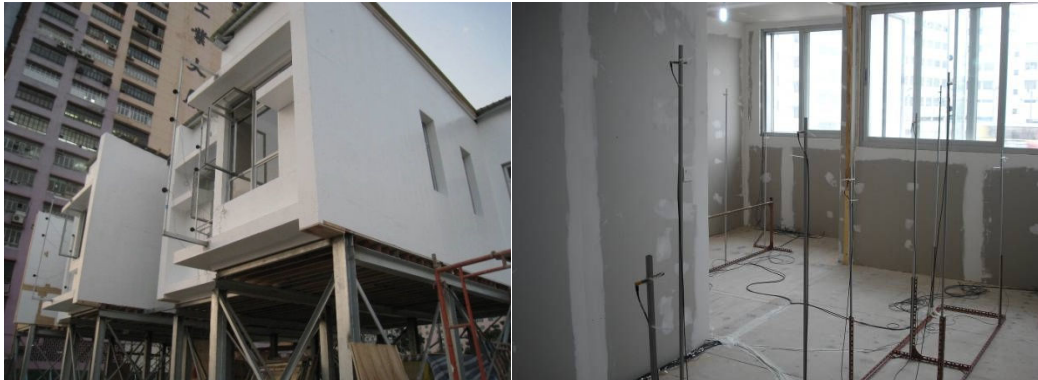
Figure 7: Microphones setup (left: façade; right: indoor)
