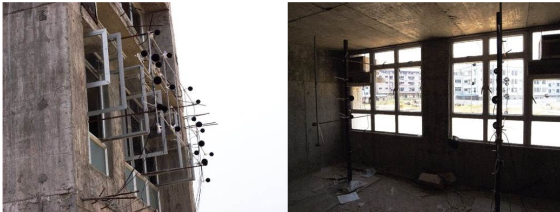
Figure 11: Microphones Setup (left: façade; right: indoor)
