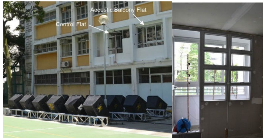
Figure 16: Mock-up Flats for Comparison of the Performance of Enhanced Acoustic Balcony and Conventional Window
