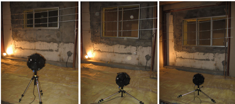
Figure 3: Laboratory Testing of Different Acoustic Window Configurations
