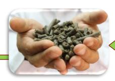
Non-Carbon material is removed & Refuse Derived Fuel (RDF) pellets are created
