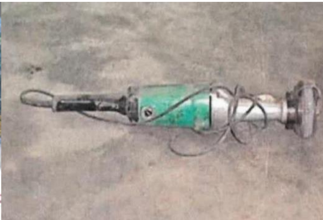
Electric grinder for night-time maintenance work in HK Tramway
