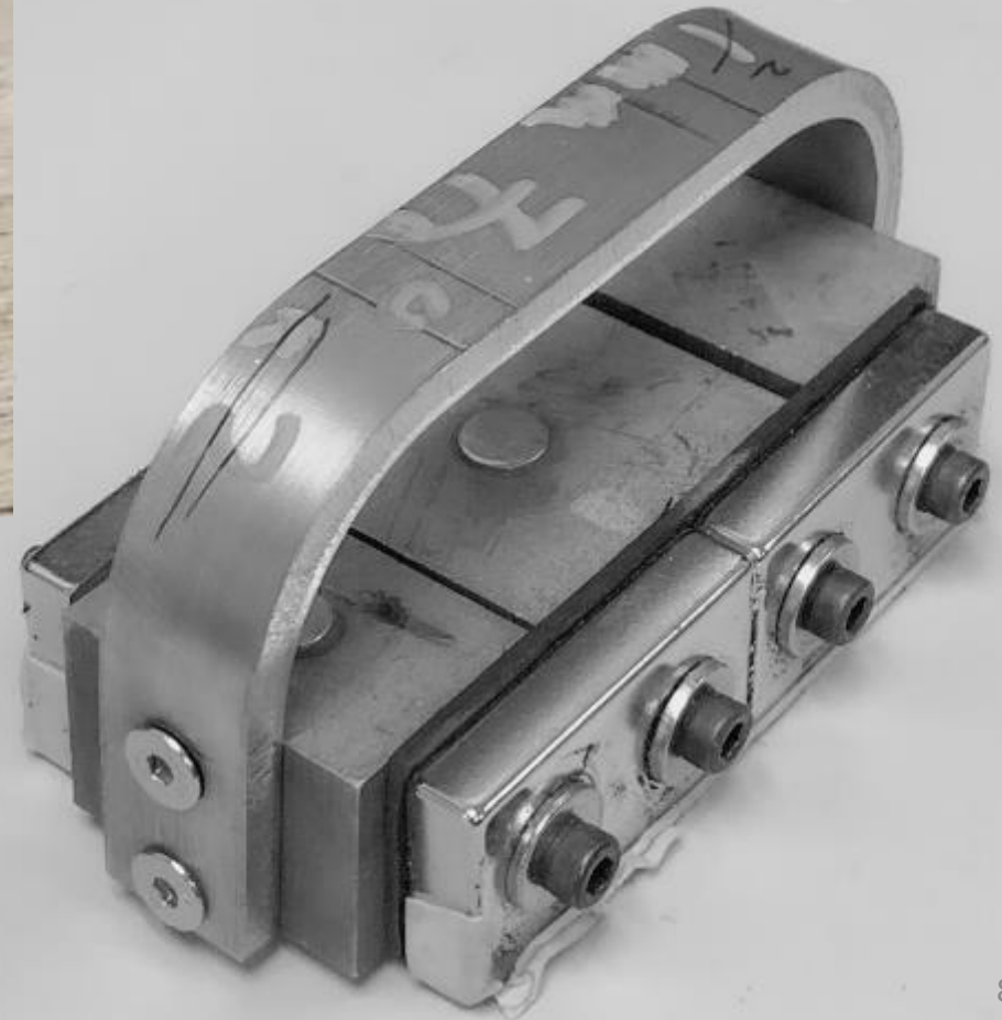
Magnetic Tuned Mass Damper used in CKR HMT (2020)
