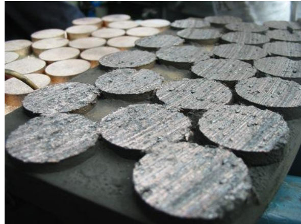
Fig. 8 Brake pads wore down to less than 5 mm
